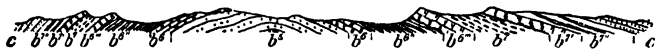
FIG 180.—Section across the anticline of Woolhope, Herefordshire. b^5 = Upper Llandovery Sandstone; b^6 = Woolhope Limestone; b^{6'} = Wenlock Shale; b^{6''} = Wenlock Limestone; b^7 = Lower Ludlow Beds; b^{7'} = Aymestry Limestone; b^{7''} = Upper Ludlow Beds; c = Old Red Sandstone.
